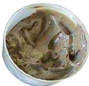
Used grease: colour turned greyish
